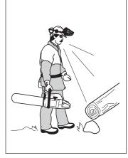
Take the utmost care when cutting through branches or logs that are in tension. A log or branch that is in tension can suddenly spring back into its natural position before or after you cut it. If you stand on the wrong side or start cutting in the wrong place it may strike you or your chain saw. This could make you lose control and cause a serious accident.
